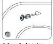
2. Remove the shipping bolts from the back of the unit.
